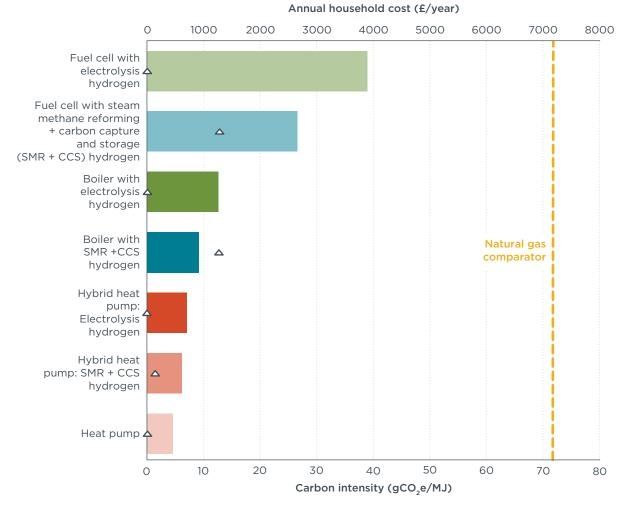
**Figure ES1:** Cost comparison and carbon intensities of different technology options for heating a typical UK single-family house for one year in 2050. Triangles represent the median values for the carbon intensity of each pathway along with a natural gas comparator.
