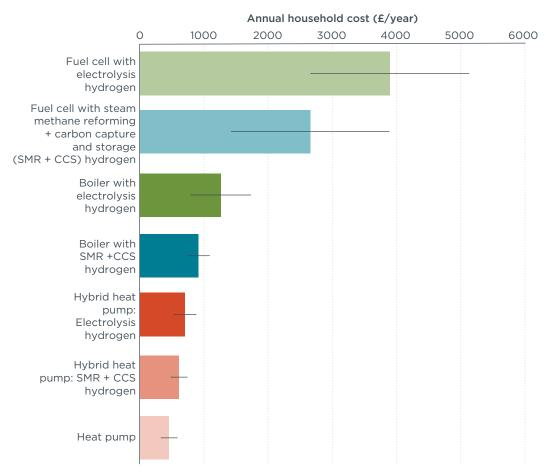
**Figure 4:** Sensitivity analysis on the cost of household heating. Error bars show the impact of varying the energy inputs (natural gas prices and renewable electricity prices) by 50%.
