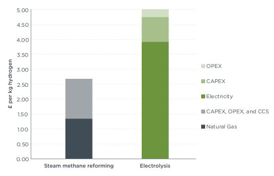
**Figure 2:** Cost components of SMR + CCS and electrolysis hydrogen prices in the United Kingdom in 2050.
