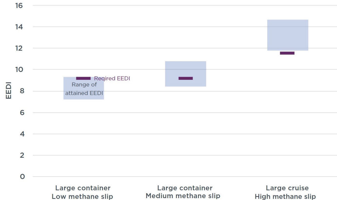
Figure 4. Potential attained EEDI of ships using LNG dual-fuel engines if EEDI were regulated on WTW CO 2 e100, accounting for a range of WTT values for LNG.
